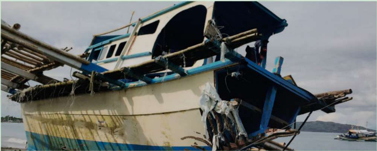
Philippine fishing vessel F/B Gem-Ver's truncated stern after being rammed by a Chinese vessel, Yuemaobinyu 42212 in Recto Bank. Photo by Department of Agriculture, 2019
